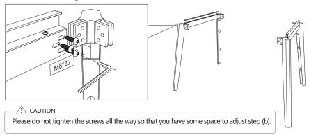
b. Plug the leg connector into the table fixture as shown below, and install the bridge connector to the base frame.
